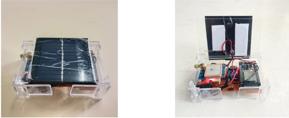
Figure 4 GPS and Pulse Sensor Module Connected to ESP32 (kit)
